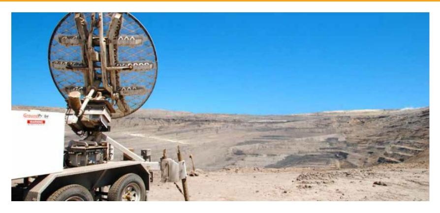
Safety is our number one priority. The Company acquired two units of Slope Stability Radar (SSR) to complement our existing Total Robotic Station for real time, 24-hour slope movement monitoring. The SSR is a state-of-the-art technology for monitoring mine walls and general slopes and is now a generally-accepted tool for high-risk slope management.
